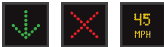
Figure 2-36. Active Traffic Management Messages
