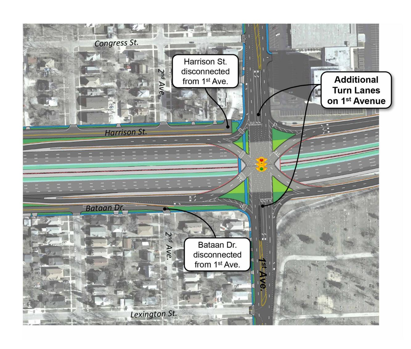
At the 1st Avenue interchange, the existing design causes long signal wait times and extensive vehicle stacking. 90% of vehicles accessing the frontage roads to or from I-290 is cut through traffic. Proposed improvements will enhance community access and improve local travel times.
