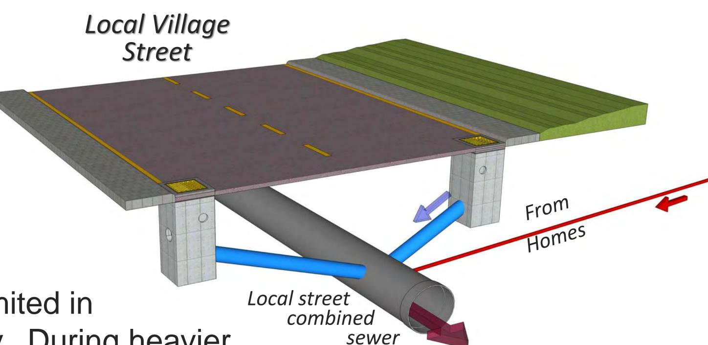
The Village sewers are limited in their conveyance capacity. During heavier intensity storm events, the runoff can flood the local Village streets and affect basements. Additionally, it also can add to the flooding that occurs to I-290.
