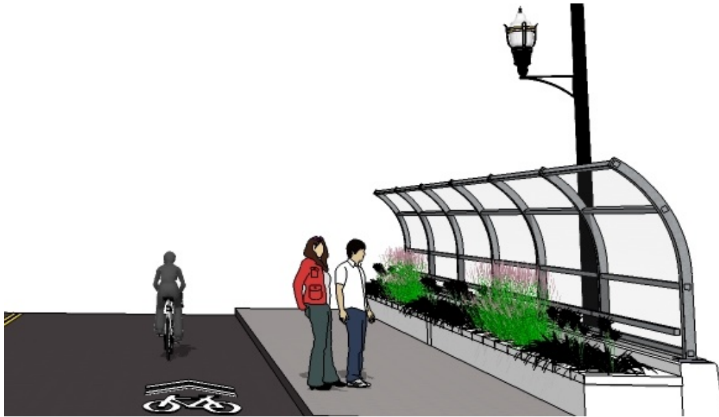
Partial Image of cross-street overpass with shared bike lane, sidewalk, planter box, lighting and safety fencing.
